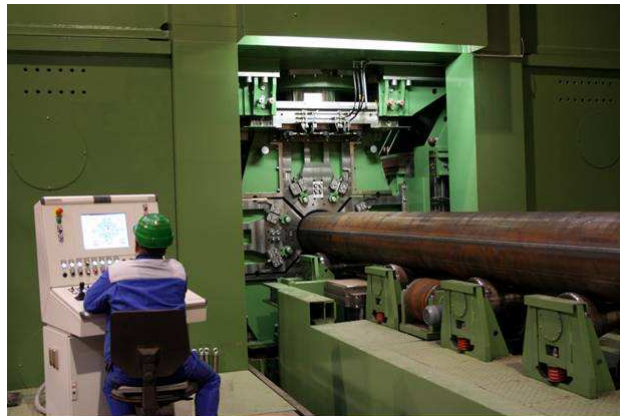
Figure 5: New calibration press called Impander®, installed at EBK in 2007
