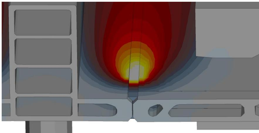
Fig. 13: Gap formation during welding of the assembly
