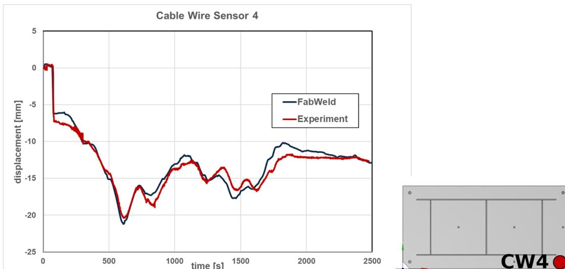
Figure 3: Validation result. Calculated deformation vs. measured deformation
