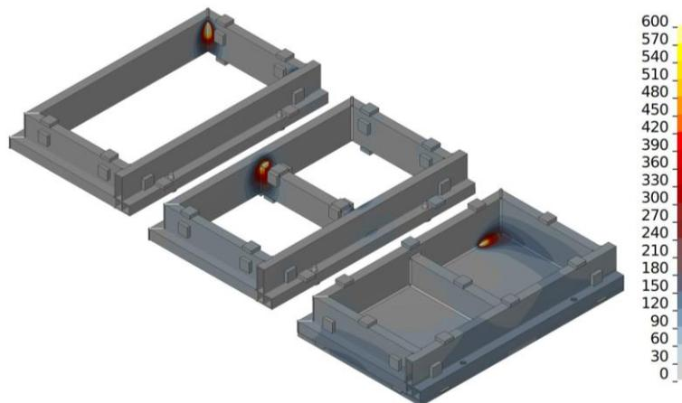
Figure 1: Multi stage assembly of welded frame structure made from Aluminium Alloys
