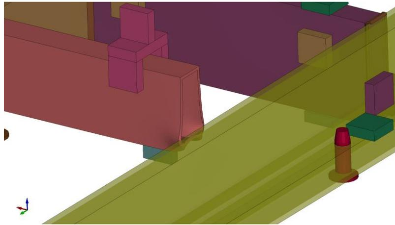
Fig. 12 Fit conflict when inserting a cross member.
