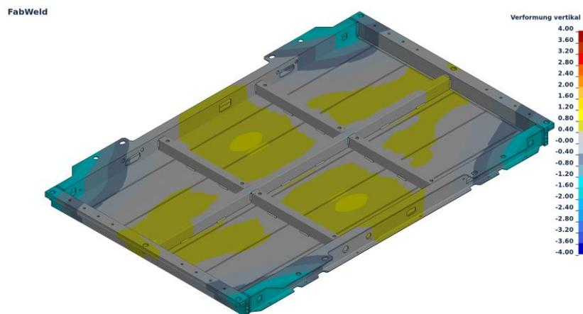
Figure 11: Optimization of variant 2, final vertical deformation
