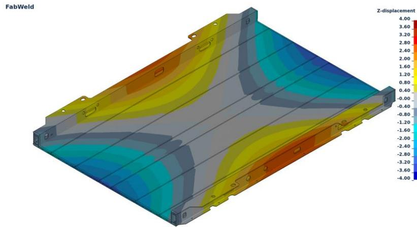
Figure 9: Vertical distortion variant 2 after station 1
