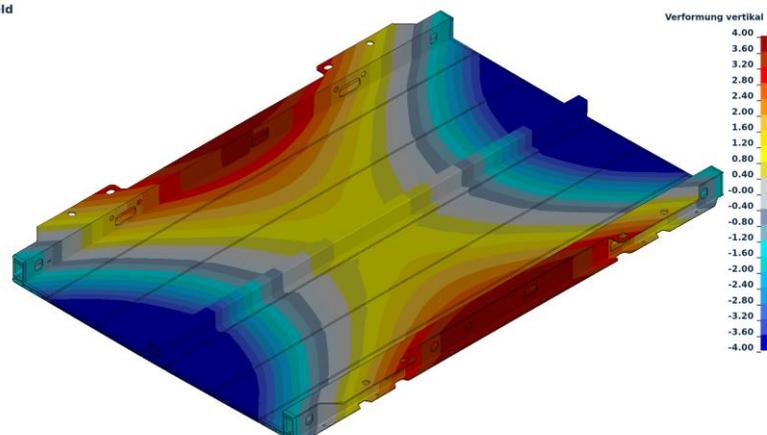
Figure 8: Vertical distortion variant 1 after station 1
